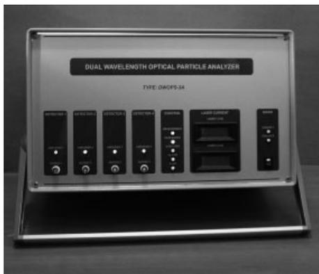
Figure 7.16 The Dual Wavelength Optical Particle Spectrometer (Analyzer) developed by Envi-Tech Ltd, Hungary.
